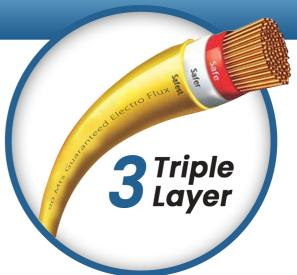
Conductors: The conductors are drawn from bright electrolytic grade copper, annealed and bunched together (multi-standed) as per class 2 and class 5 of IS 8130:2013
